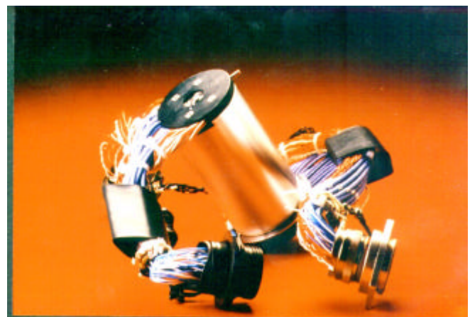
Figure 2: Slip Ring used in Military Vehicle Commander's Viewer
